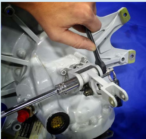
Vector Aerospace maintenance on H130 Tail Rotor Gearbox in Richmond BC Photo: Vector Aerospace
