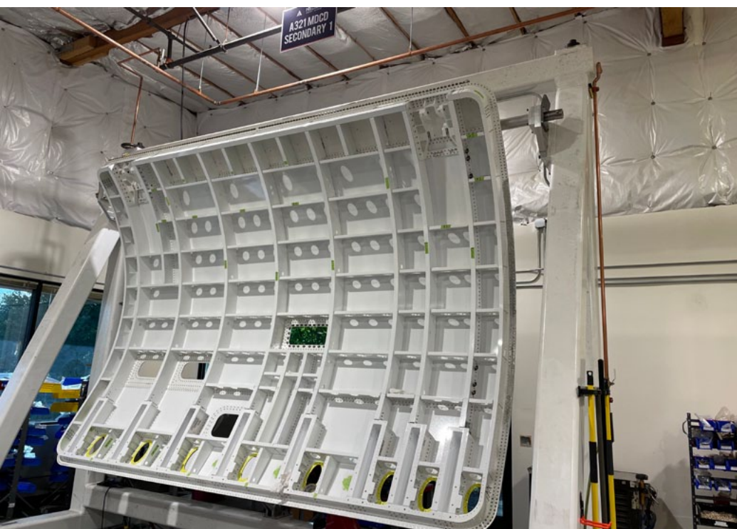
Cargo door during the conversion process. Photo: 321 Precision
