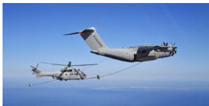
A400M performing dry contacts with an H225M operated by Airbus Helicopters Photo: DGA Essais en vol
