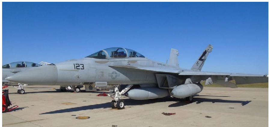
An F/A-18 Super Hornet equipped with a Block II Infrared Search and Track prepares for its first flight with the long-range sensor Photo: Boeing
