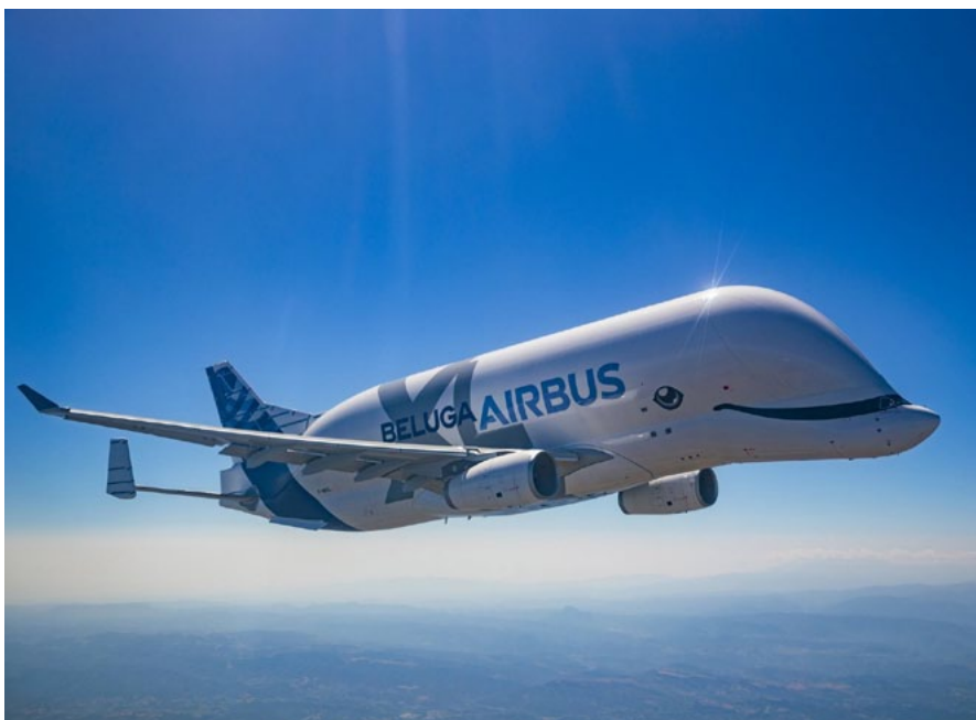
The BelugaXL has the largest cargo bay cross-section of all existing cargo aircraft worldwide
