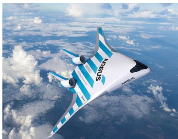
Airbus has revealed MAVERIC (Model Aircraft for Validation and Experimentation of Robust Innovative Controls) its "blended wing body" scale model technological demonstrator
