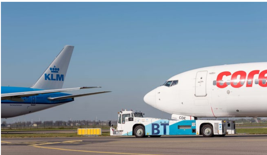
Aircraft taxiing with the TaxiBot at Schiphol Airport
