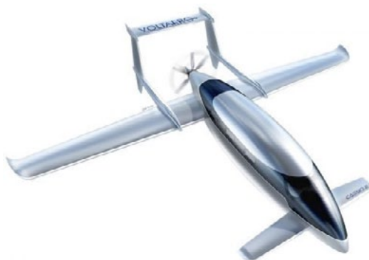
The production Cassio aircraft has a sleek, aerodynamically optimized fuselage with a forward fixed canard and an aft-set wing with twin booms that support a high-set horizontal tail Photo: VoltAero
