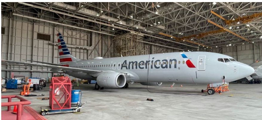
After 12 days in the paint shop, American’s first 737-800 to be repainted with Silver Eagle non-mica paint is ready for departure Photo: American Airlines
