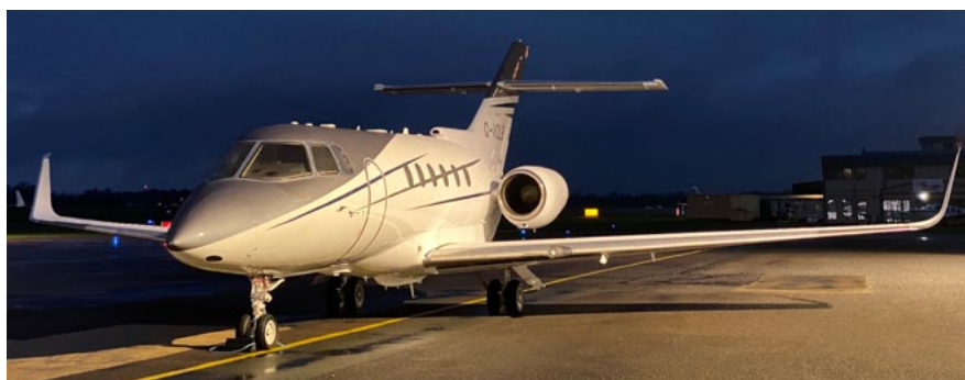
Hawker 800XPi airplane Blended Winglet retrofit
