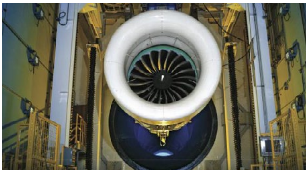
P&W Geared Turbofan™ PW1100G-JM engine testing at the West Palm Beach Engine Center in Florida Photo: P&W
