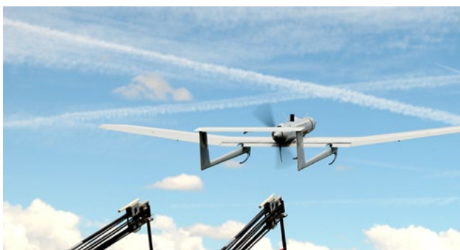
Launched by catapult, the Aliaca maritime UAS concludes its flight by landing automatically using a dedicated net landing solution
