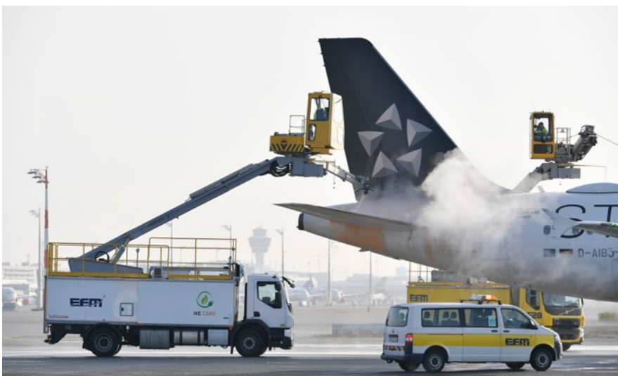
The de-icing vehicle can complete about two to three hours of operation and thus de-ice about 10 to 15 aircraft Photo: Munich Airport
