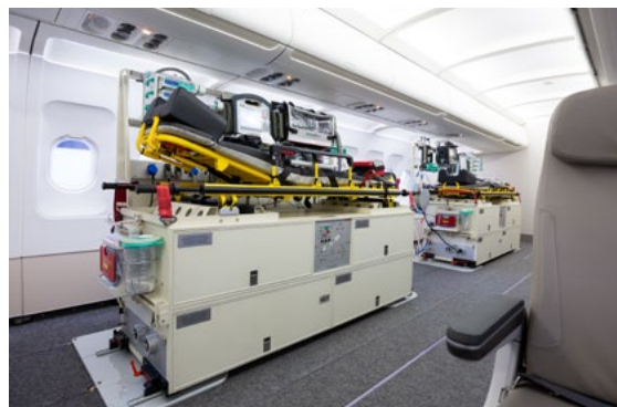
The first-generation PTE, here seen installed in an Airbus A319 Photo: LHT
