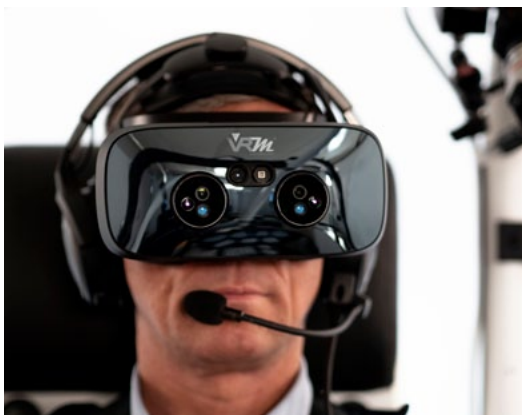
Virtual Reality (VR) based Flight Simulation Training Device (FSTD), developed by VRM Switzerland Photo: EASA
