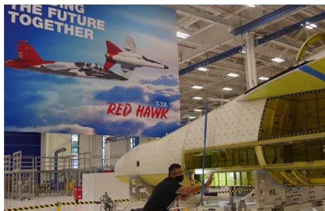
Boeing T-7A Red Hawk aircraft mechanic examines the surface of the first spliced advanced trainer being produced in St. Louis Photo: Boeing
