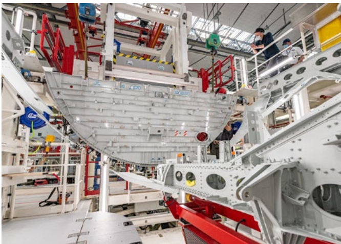
Production has started in Germany with the structural assembly of the center and rear fuselages for the A321XLR Photo: Airbus
