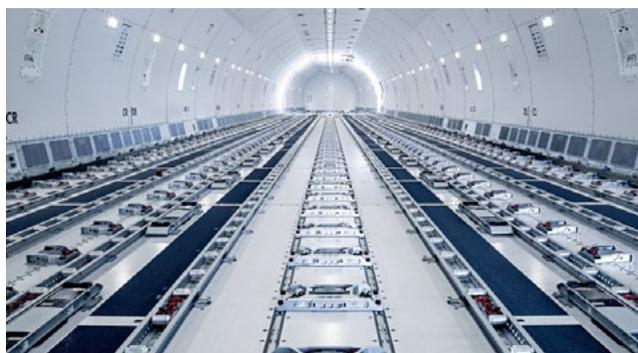
The Boeing 777F has a standard payload capacity of 103 metric tons
