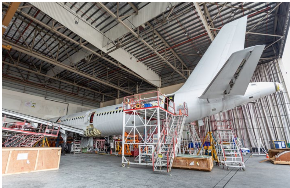
Airbus A321P2F undergoing cargo conversion
