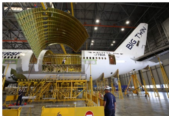
Door cutting in the hull to install a cargo door
