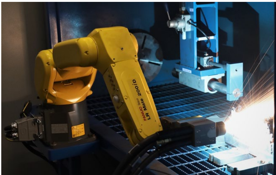
Photo: Fokker Services has installed new Twin Wire Electric Arc Spray technology at its LaGrange, GA, USA facility
