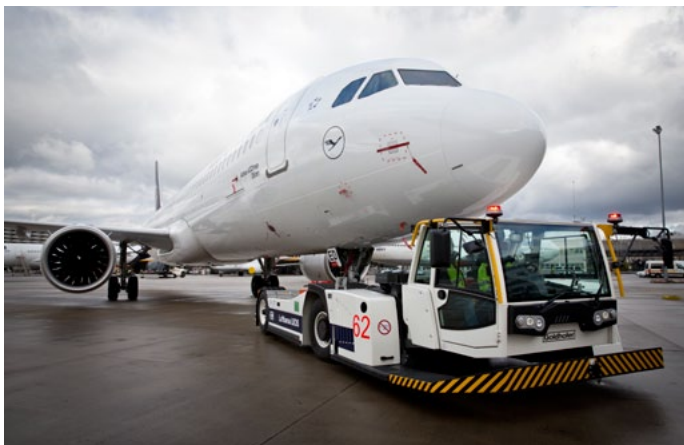
The all-electric towbar-less aircraft tractor Phoenix E is operating for Lufthansa LEOS Photo: Lufthansa
