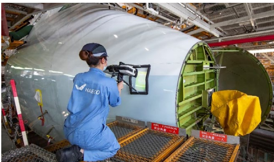
Photo: HAECO Group is using 8tree's dentCHECK tool to enhance the efficiency and quality of its dent-mapping activities
