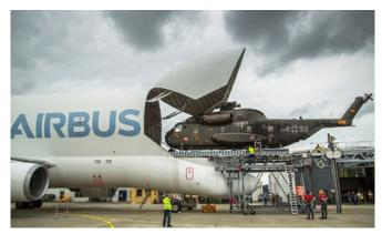
Lifting of a CH53 military medium-lift helicopter into the Beluga
