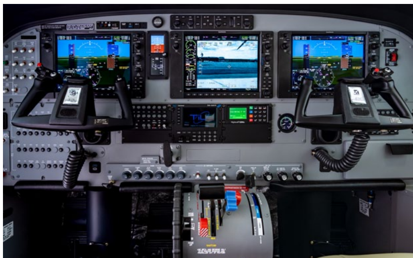
Electronic flight instrument system (EFIS) on Cessna 208 Caravan
