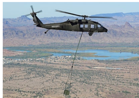
Uninhabited Black Hawk® helicopter lifts external cargo Photo: Sikorsky
