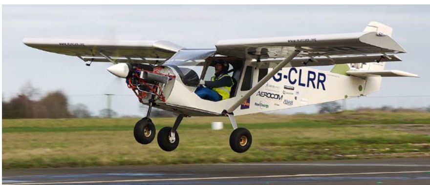
The 'electric sky jeep', based on a Zenith CH750 aircraft
