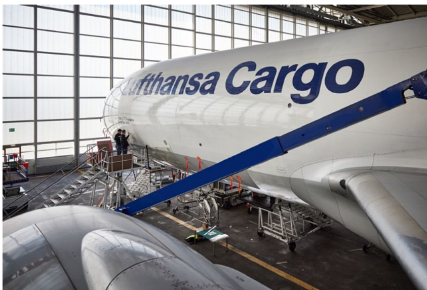
Modification of Lufthansa Cargo's first 777F with AeroSHARK
